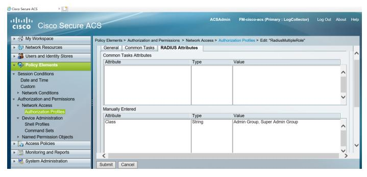
Figure 6 Supplying the Class Field for RADIUS (ACS 5.x)
