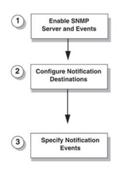
Figure 36 Configuring SNMP Notifications
